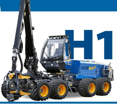
Service weight from 17 400 kg (6WD) / 18 900 kg (8WD) Lenght 7 938 mm Width 2 830 mm Transportation height 3 591 mm Ground clearance 600 mm
