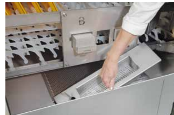
Only a few parts need to be removed for daily cleaning.
