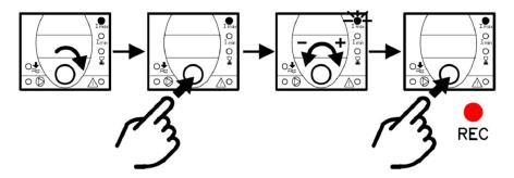
How to change the thermal underload protection  $(I_{min})$
