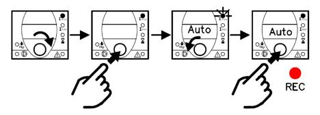
How to change the thermal overload protection (I<sub>max</sub>)
