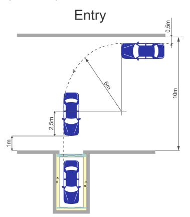
Vehicle lift VL45 has larger cabin and wider doors. Minimum distance of 8,5 m should be sufficient.
