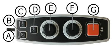
The unit can be used in simple profile or advanced profile. When the unit is in simple profile the LED lights green. When the unit is in advanced profile the LED lights blue. There is also a settings mode. When the unit is in settings mode it lights yellow.
