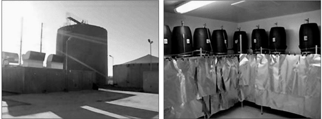
Figure: Batch fermentation (container-scale and laboratory-scale) (Photo: Fachverband Biogas e.V., University of Rostock)
