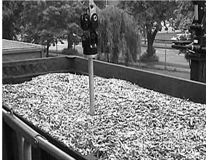
Figure 4: NIR prob for measurement of moisture content (photo: Bestwood)
