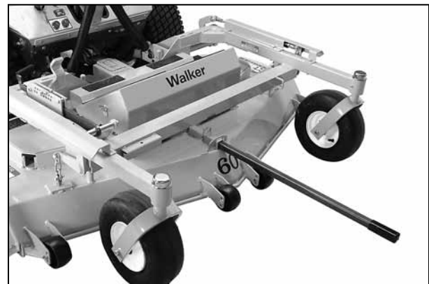
Tilt Bar Installed
