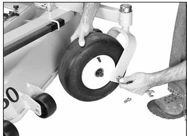
Deck Caster Wheel Installation
