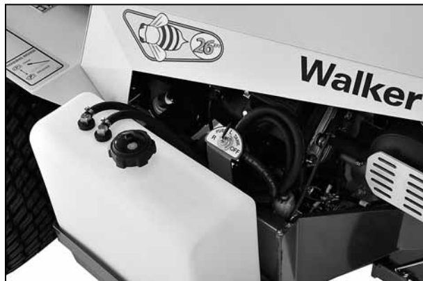
Fuel Selector Valve - Model MBS26
