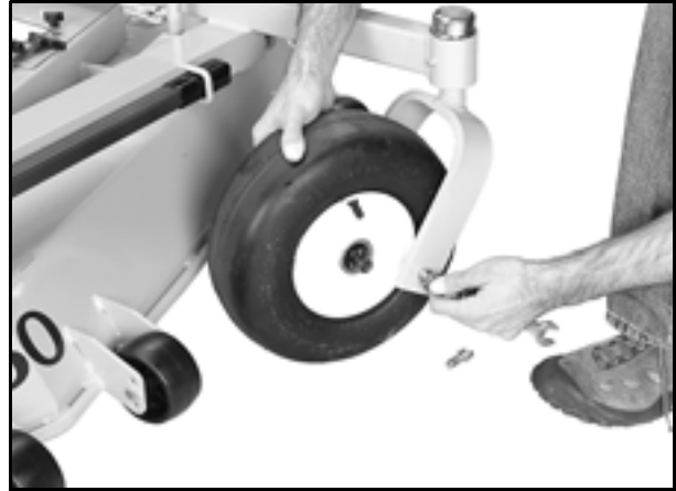
Deck Caster Wheel Installation
