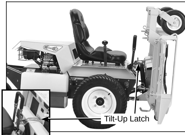
Deck Secured in Tilt-Up Position
