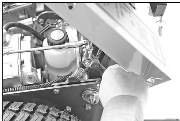
Stop Bolt Adjustment
