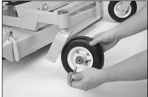
Deck Caster Wheel Installation
