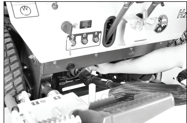
Coupler Installation Tool Removal
