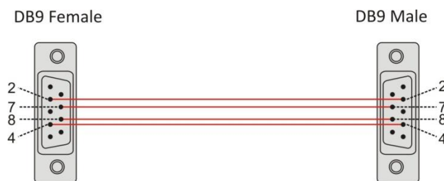
Fig. 26 – Building an extension cable
