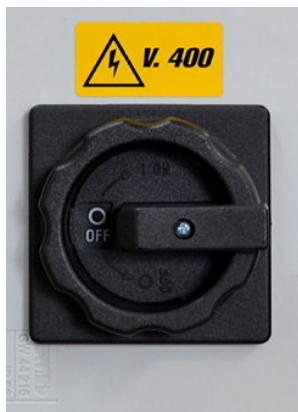
Fig. 17: Switch on the machine
