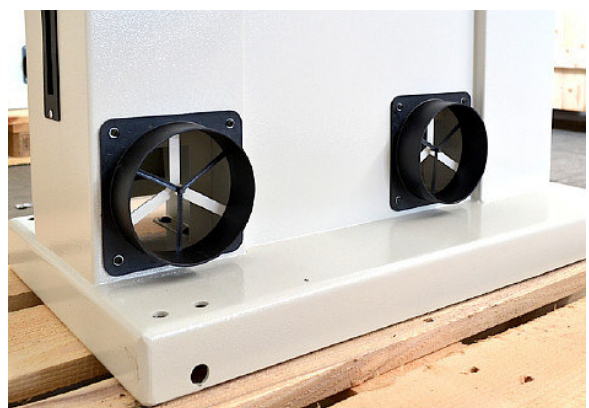
Fig. 8: Connection exhaust system
