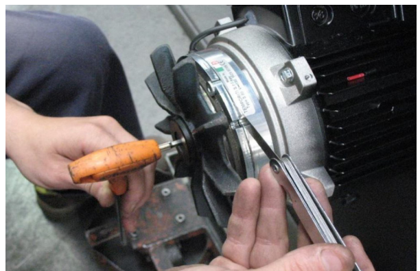
Fig. 30: Maintain gap width (0.2 mm)
