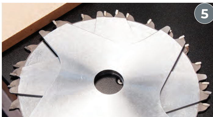
Find a scrap piece of timber the thickness of the cut as a guide. Place the inner blade against the timber and start stacking the chipper blades on top. Make sure the teeth are spaced equally and pointing forward.
