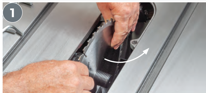
Make sure the teeth of the inner and outer blades are facing inward.
