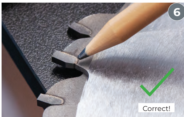
Find a scrap piece of timber the thickness of the cut as a guide. Place the inner blade against the timber and start stacking the chipper blades on top. Make sure the teeth are spaced equally and pointing forward.
