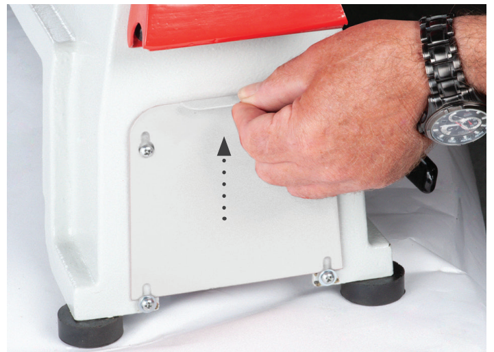
Lower motor pulley access plate
