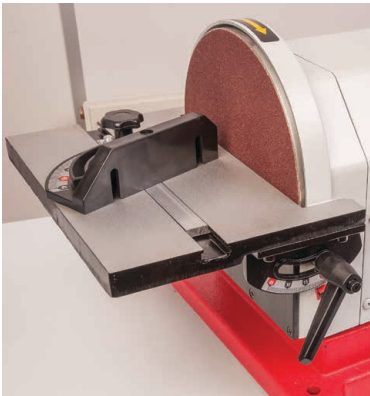
Sanding disc table set at 90° degrees
