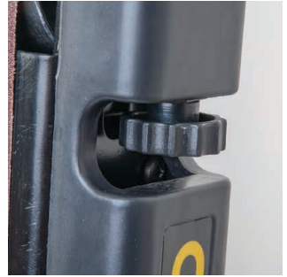
Linisher belt tracking control wheel
