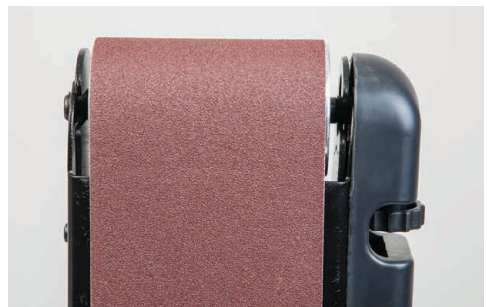
Belt running down the centre of the linisher
