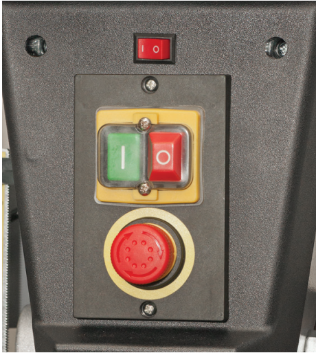
AP32FD pillar drill control panel NOTE: The LED light switch is above the On/Off switch assembly
