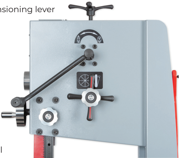
Upper blade guide clamp Tracking control knob Tracking control lock
