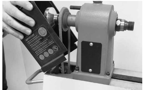
Lower the headstock cover to reveal the pulley system
