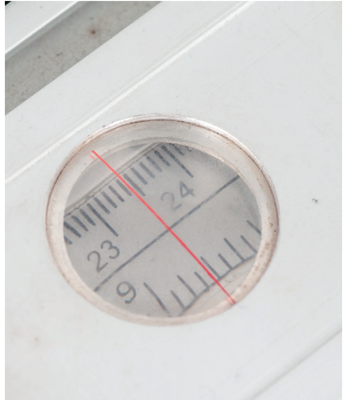
Rip fence magnifying glass and index marker
