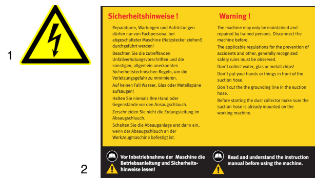
Fig. 1: Safety labels: 1 Warning of dangerous electrical voltage | 2 Safety instructions
