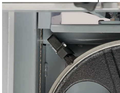
Lower saw wheel brush (upper)
