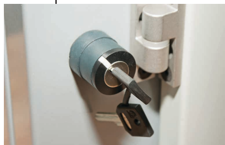
The electro-magnetic brake switch, set to the 'OFF' position isolating the bandsaw
