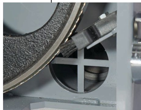
Lower saw wheel brush and dust extraction outlet
