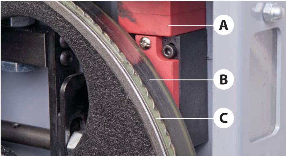
Micro switch (A), Blade (B), Tyre (C)
