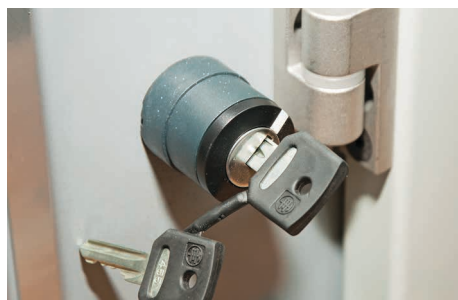
The electro-magnetic brake switch, set to the 'ON' position
