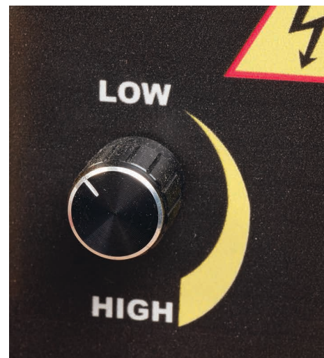
Variable speed control knob 250-3,550rpm
