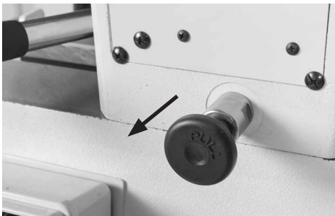
Headstock Pivot Lock, pull this knob to rotate the headstock to the desired position
