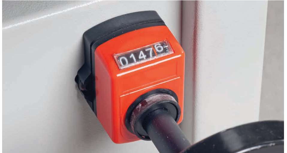
The Digital Thickness Display, will give an accurate visual indication of the amount you are adjusting the thickening table in 0.10mm increments.
