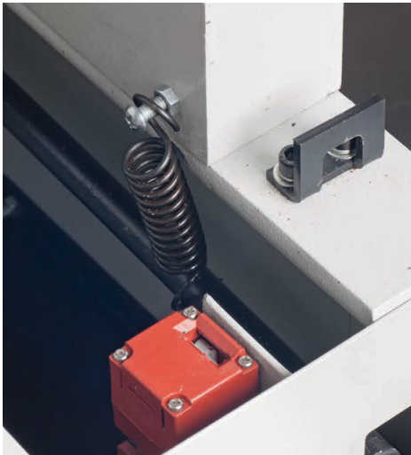
Thickener cover safety micro switch
