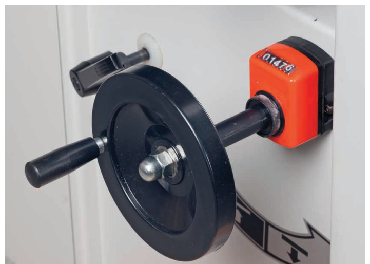
Thickening table rise and fall control wheel
