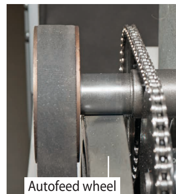
Autofeed wheel engaged
