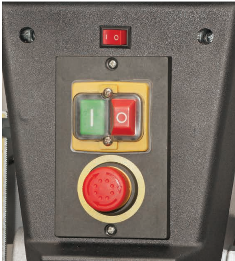
AP540PD pillar drill control panel NOTE: The LED light switch is above the On/Off switch assembly
