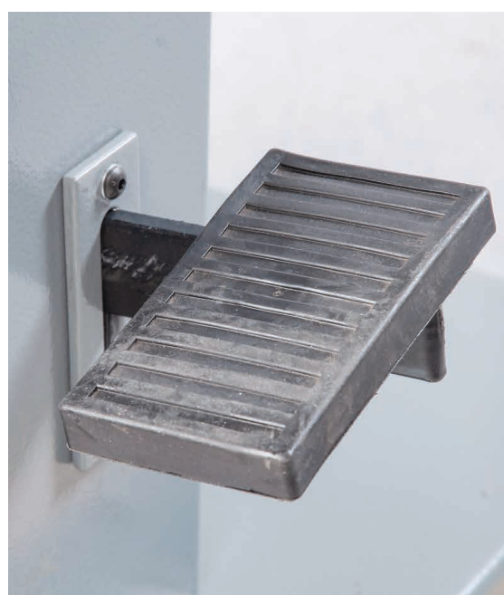
Corner peddle foot brake stop Press down to stop the bandsaw instantly
