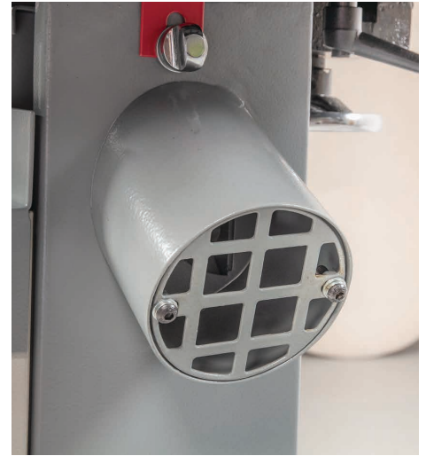
Dust extraction outlet
