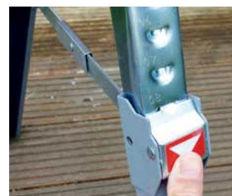
With a choice of eight settings, outer legs are simply slid downwards and locate in notches at 27mm intervals
