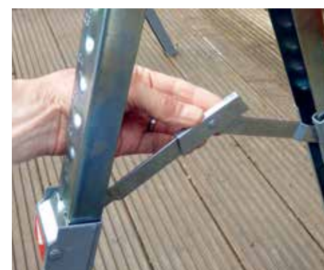
A hinged cross-brace locks the legs apart, then you can adjust working height
