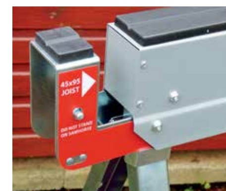
What makes each sawhorse clever is the cut-out at each end for a piece of 95 x 45mm softwood
