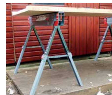
Once stretchers are in place, you have a rigid, pop-up work surface
