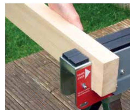
Use CLS timber (which finishes at around 43mm), to achieve a tight fit into the slot
