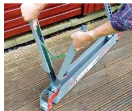
Depressing a spring-loaded button at one end of the rail enables you to unfold the first pair of legs
