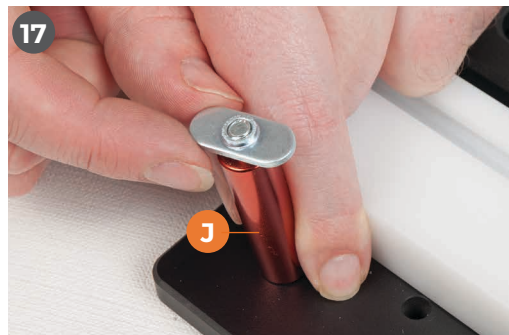
Locate the four oval nuts you removed earlier and reattach as illustrated
