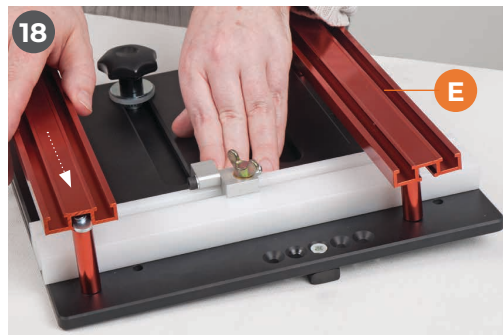
Line up the oval nuts in the height spacers (J) with the 'T' slots in the guide rails (E) and slide the guide rails on
